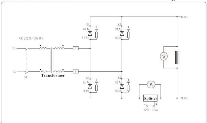
Feedback isolated full control bridge style rectifier wiring
